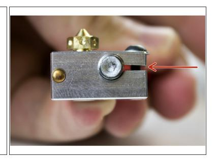
• Tighten the M3 x 10 socket dome screw (with the M3 washer on it) with 2 mm hey key until the clamp deforms slightly (as shown in the second picture).
