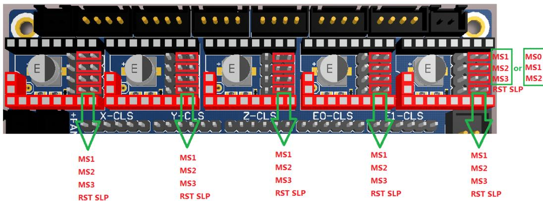
Note: if you are using A4988 or DRV8825 driver, you must connect RST and SLP with jumper cap.
